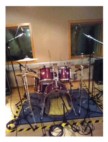
The overheads will be formed into a standard spaced pair (A/B pair) to capture the drum kit in a natural way. Spaced pairs can cause phase issues typically because of the distance between the instrument and sound source. To avoid this I can follow the 3:1 rule where mics are spaced away from each 3x the amount mic A is from the sound source.
