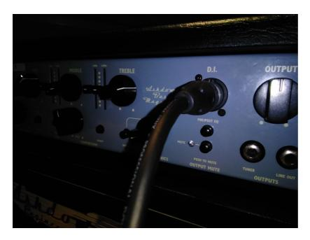
For this particular bass amp (Ashdown MAG-C210) there is no mic required as it has a built-in DI and output which can be cabled directly into the xlr wallbox for the mixing desk.
