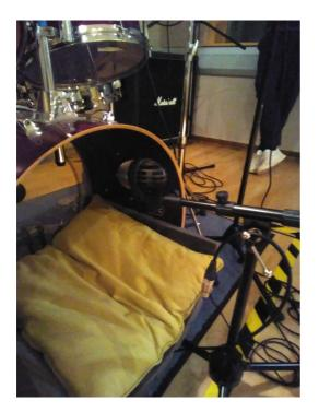
Kick drum is close mic'd with a cardioid dynamic microphone pointed to the center of the outer skin to capture a clean transient and low end thump.
