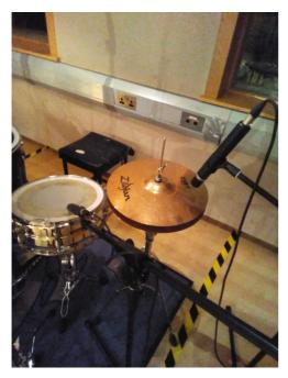
Snare – The mic is structured horizontally with the mic facing inwards towards the center of the skin to capture the initial transient hit and less of the surrounding rumble from arround the snare.
