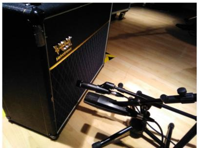
The electric guitar will be close mic'd with the dynamic mircrophone pointed directly at the center of the amps speaker to capture the pure direct tone of the amp.
